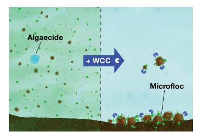
Diagram shows improved water clarity and augmented floc formation after REGEN-Clarify® application.
