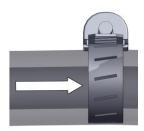
Slide tubing clamp over tubing and barbed portion of the fitting. Tighten clamp using a socket/nut driver or flathead screwdriver.
